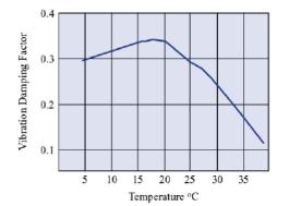
The vibration damping performance of a material can be defined by its 'damping factor'.
